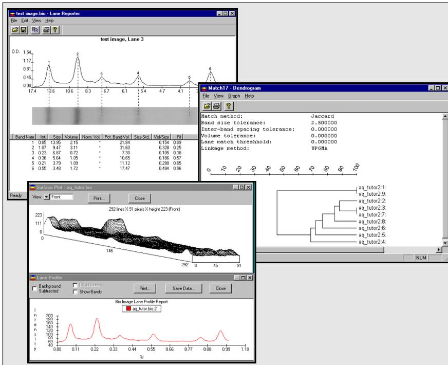
Advanced Quantifier software lets you quickly and reproducibly analyze protein or DNA samples run in one-dimensional separations. The software automatically locates lanes and bands. On command, it determines band size and quantity of sample present in comparison to standards or reference lanes.
